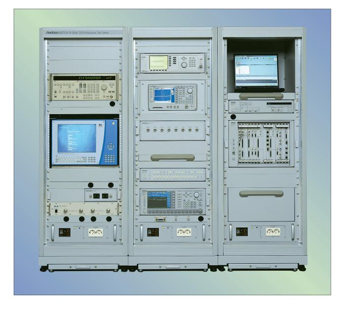
Testing System Conforming to Clause 5, 6, 7 in 3GPP TS34.121 Standards
